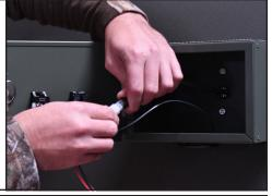
9. Connect and install battery into the Power Shelf.
