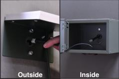
8. Connect Solar Panel to wiring harness inside the Power Shelf.
