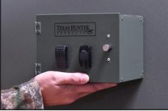
3. Open access panel and mark position of top, bottom and center holes.
