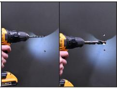
5. Install Power Shelf with the two 1/4" x 3/4" bolts supplied in solar panel packaging. For walls thicker than 1/4", you will need to obtain longer bolts - 1/2" longer than the thickness of the wall.
