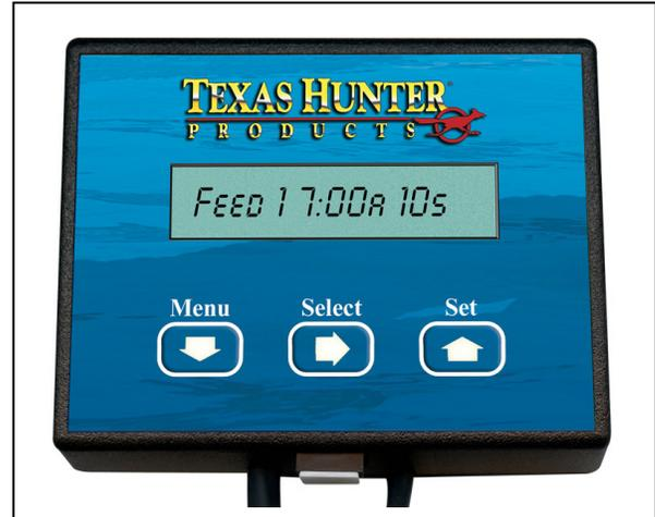
**1. Connect the Battery.** Important: This feeder requires a 12-volt rechargeable battery to ensure proper motor function. Connect the Positive (+) Red wire and Negative (-) Black wire to the battery. Press **Menu** button twice to display Battery condition.
