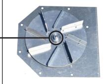
5. Using an 11/32" or 7mm socket, open-end or crescent wrench, remove the two motor bolt nuts. Remove the other half of the blower assembly from the motor.
