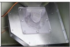
2. Remove the 12 screws on front of feeder where the feed comes out. Unplug motor and remove blower assembly.
