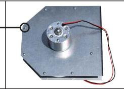
4. Using the 5/64" Allen wrench, loosen the set screw on the motor hub and remove the Impeller Wheel.
