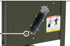
3. Remove the 7 screws on the motor side of the blower assembly to dis-assemble the two halves of the blower assembly.
