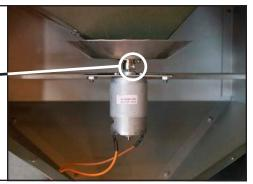
9. Run wires through small hole in funnel. Install plug on end of wires, plug is color coded to wire color.
