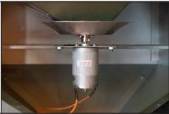
8. Tighten cup spinner plate set screw, using gap measurement from Step 4 between bottom of funnel and cup spinner plate. Should be about 3/8".
