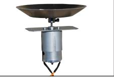
7. Install new motor, small rectangular bracket, and spinner plate on motor bracket that goes all the way across funnel using nuts from Step 3.
